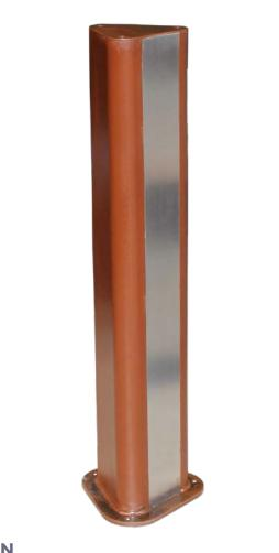
Design bollard model Trian built by a triangularshaped structure in cor-ten steel cylinder plate. Great thickness for greater rigidity, varnished to prevent future corten oxidation and decorative satin stainless steel front plate. All on corten steel anchor plate also triangular in shape, with three holes to fix to the pavement.
