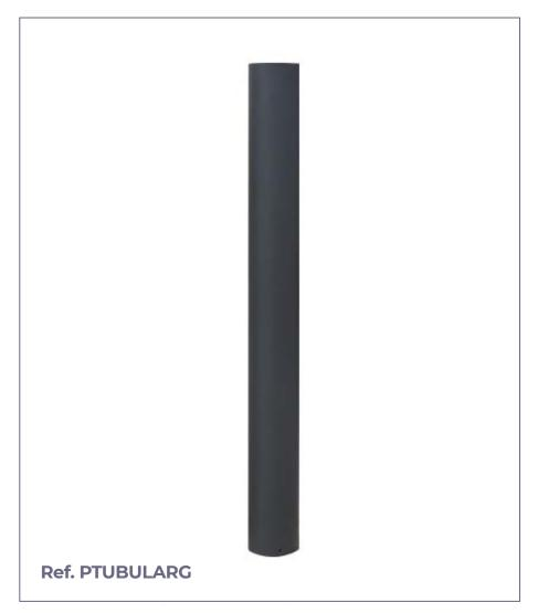
Tubular bollard model built with galvanized iron tube with a diameter of ø 95 or 220 mm. and 2.5 mm. of thickness. Total height of 1000 mm.
