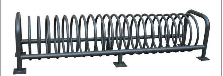
**Twister model bicycle rack set,** built in galvanised iron for 20 bikes. Manufactured from a Ø 450 mm curved tube with a Ø 25 mm diameter tube and welded on a Ø 48 mm tube structure with anchor plates to be fixed by metal plugs.
