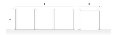
Universal bike parking made out of galvanised, 304 stainless, or weathering steel.
